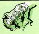
BALL-GEAR STEERING utilizes scores of polished steel balls to minimize friction and keep steering light yet firm for easy handling. Standard equipment, all models.
