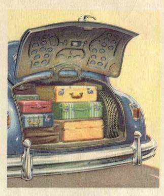
The counter-balanced rear deck lid raises and lowers with little effort. Will remain open with no danger of it falling shut. Extra large storage compartment in the rear deck of all body styles.
