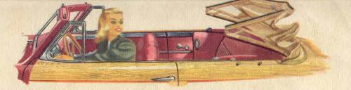
To raise and lower the Convertible Coupe top, you merely release the locking device and turn the Switch on Instrument Panel. The top folds back, quickly and compactly into a recess behind the rear seat.
