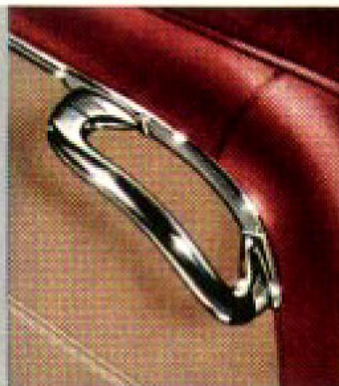
Chrome-plated assist handles are securely mounted on each side of the back of the front seat to facilitate getting in and out of the car—an important safety feature.
