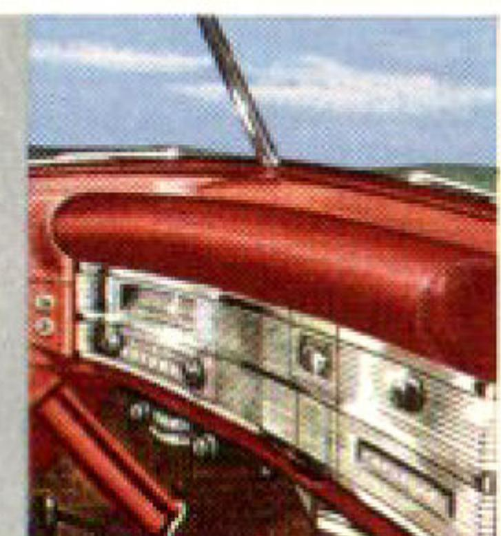
The Chrysler Safety Cushion, extending across the top of the dash panel, is made of thick sponge rubber and covered with leather—a great safety feature.
