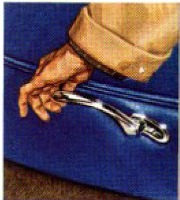
Lift the handle on the left side of the front seat and the seat can be moved forward quickly and easily to exactly the most comfortable and convenient position.
