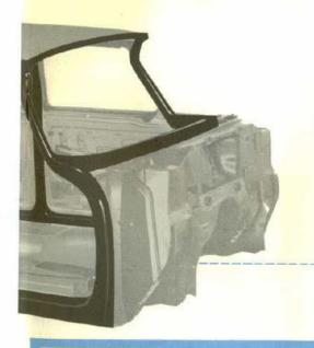
Herculite door glass—three times stronger than laminated glass! A Plymouth taxicab exclusive! Resists cracking or breaking no matter how hard and often the cab doors are slammed! Plymouth pioneered its use in taxi doors—to keep your cabs from layup time for broken glass replacement! A big saver of time and money!
