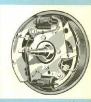
TOTAL CONTACT BRAKES, with new advanced step design—a Plymouth exclusive in the taxi field, are especially adapted to taxicab stop-and-go driving because the brake shoe follows the wheel drum as the drum expands from heat, maintaining safe stopping contact. Each front wheel has two brake cylinders. Stops are safer and surer, with 25% less pedal pressure. Plymouth brake linings are bonded to shoe... no rivets to score drums.
