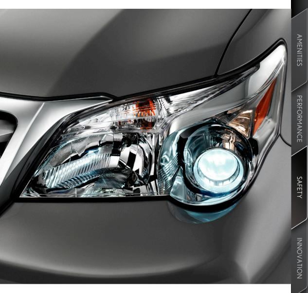
When you're rounding a turn in the dark, unidirectional headlamps that illuminate the area adjacent to the curve aren't nearly as effective as the advanced Adaptive Front Lighting System available on the GX. It can help illuminate the road by rotating the right headlamp up to 10 degrees and the left headlamp up to 15 degrees into a turn.
