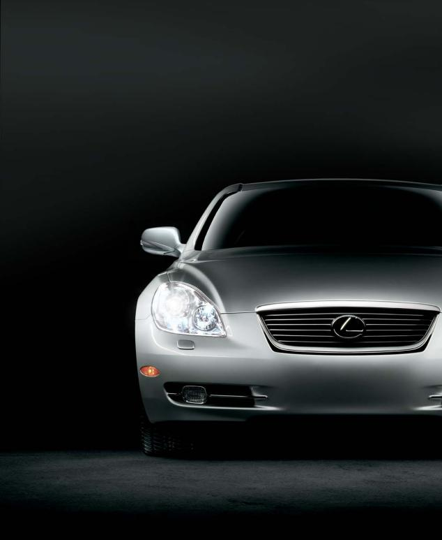
While the jeweled-cluster headlamps on the SC are attractive in their own right, they actually serve a purpose. To help illuminate more of the road through turns, the Adaptive Front Lighting System (AFS) can pivot the left headlamp up to 15 degrees and the right headlamp up to 5 degrees into a curve. And to help reduce glare to oncoming traffic, dynamic auto-leveling High-Intensity Discharge (HID) headlamps automatically sense and adjust to changes in load and road conditions.
