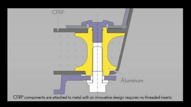
The LFA team also developed an advanced joining technology to bond carbon fiber and metal components. Conventional joining processes use a threaded aluminum insert that is wrapped in the CFRP. However, the LFA uses an innovative system that required no insert or direct CFRP contact by employing a flanged aluminum collar to link the two materials, overcoming inherent weaknesses in such joints.
