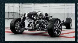
All-new front and rear suspensions were engineered with aluminum components, reducing unsprung weight and delivering significantly greater agility. In the rear, improved suspension geometry further enhances control and tire cornering force. Learn more at lexus.com/GS/platform.
