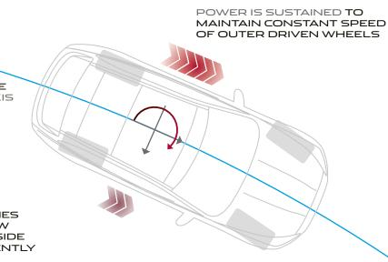
ADDITIONAL ROTATIONAL FORCE APPLIED AROUND VEHICLE'S AXIS
