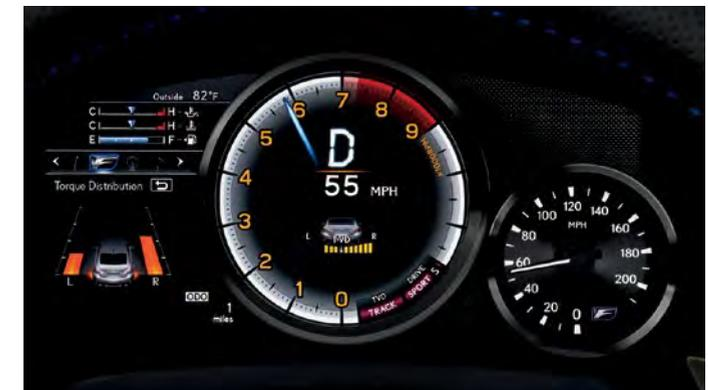
For added agility, the RC F offers a Torque Vectoring Differential. Designed to improve performance with three driver-selectable modes—Standard, Slalom and Track—it can respond in one-thousandth of a second to vary torque distribution according to cornering conditions. By sending more power to the outside rear tire, it helps propel the RC F around turns for enhanced agility, while helping you to hold your line with ultimate precision.
