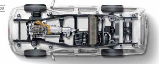
28 HYBRID POWERTRAIN The Two-Mode Hybrid System saves fuel with an all-electric launch, low-speed electric-only propulsion and electric assist during demanding driving. It is comprised of a Vortec 6.0L VVT V-8 engine, two 60-kilowatt electric motors housed within the transmission that also act as generators, a 300-volt battery that powers the system and an innovative regenerative braking system that results in an EPA-estimated 20 mpg city/23 mpg highway for both Sierra and Yukon.
