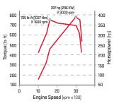
Duramax Diesel 6.6L V-8 Horsepower & Torque • SAE Certified
