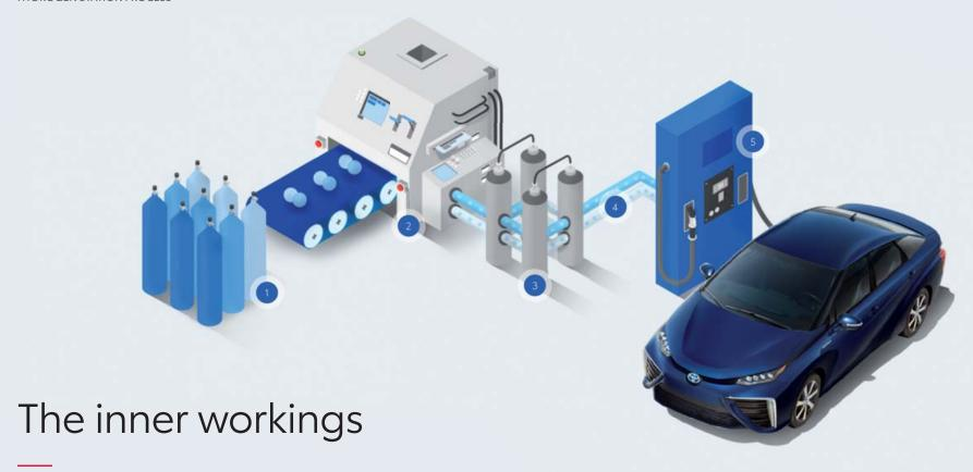
Hydrogen stations take processed hydrogen, compress it and cool it to deliver it safely to your Mirai. Since the equipment is built above ground, it is safe and easy to install, service and upgrade.
