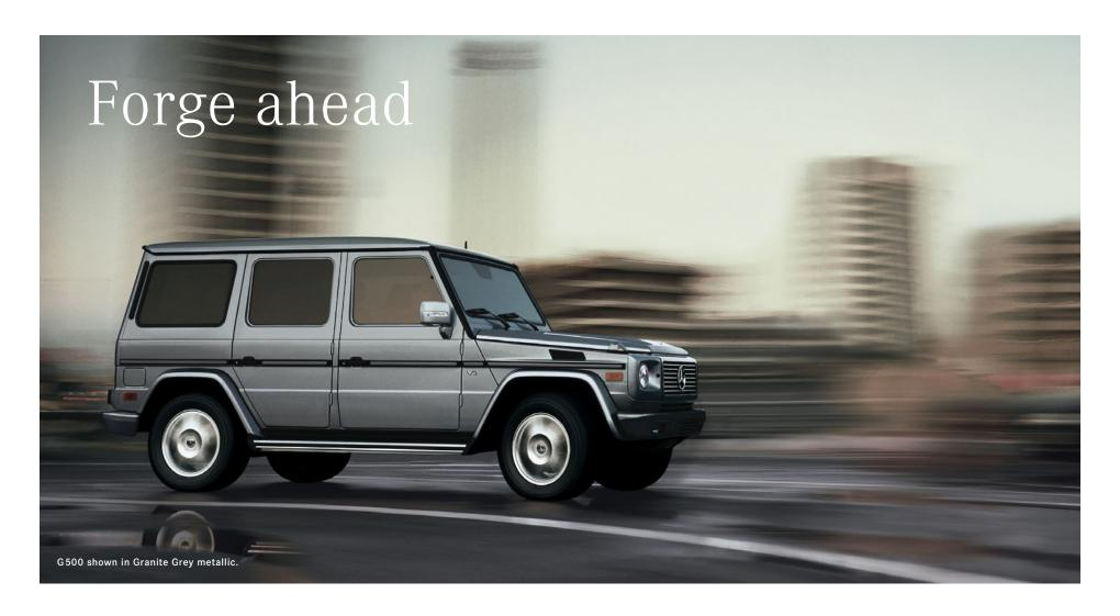
Blaze your own trail in the unique, hand-built G 500. A massive 292-hp 5.0-liter V-8 delivers a robust 336 lb-ft of torque and more than enough motivation to escape the ordinary. Power is applied through an advanced driver-adaptive 5-speed automatic transmission that adjusts its shift points to match your driving style. The Touch Shift
