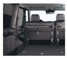
Here's one standard feature that actually gives you options. The second-row seats fold forward in a 60/40 split, so you can accommodate up to five passengers, or nearly 80 cu ft of cargo, or a variety of combinations in between.
