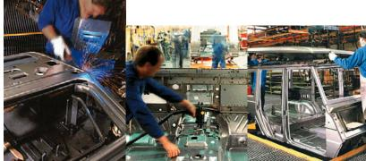
Life for the G-Class begins in the inspired hands of its craftsmen. In fact, from the very first weld, each craftsman signs off on his or her part of the process. An extremely rigid steel frame is constructed using fully boxed longitudinal rails and six tubular crossmembers to further enhance torsional stiffness.
