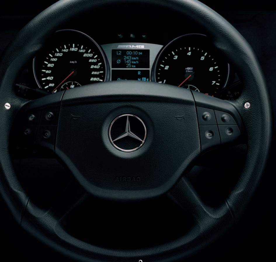
2 gearshift buttons on the AMG ergonomic sports steering wheel and the AMG instrument cluster with specially adapted multifunction display menu – including a racetimer, engine oil temperature gauge and central gear indicator
