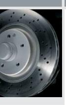
To match the impressive power of their V-6 engines, the SLK 280 and SLK 350 have equally impressive braking systems. Large ventilated front rotors – 13.0" on the SLK 350, 11.8" on the SLK 280 – help reduce brake fade in even the most vigorous situations. On the SLK 350, the front rotors feature perforations to help divert water, dirt and heat away from the brake components. Dual-piston front calipers were chosen for the SLK 350 because of their ability to apply stronger brake forces across the
