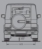
The dimensions shown are mean values (in mm) and apply to standard-specification vehicles carrying three occupants weighing 68 kg each
