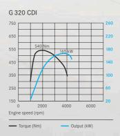
G 320 CDI. The 3-litre V6 diesel engine achieves its maximum output of 165 kW (224 hp) at just  $3800\,\mathrm{rpm}$
