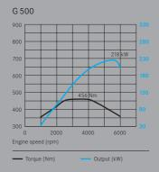
${\bf G}$  500. The G 500 achieves its peak torque of 456 Nm across a broad engine speed range from 2800 rpm to 4000 rpm
