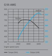
Full power ahead. The impressive torque of 700 Nm is available across a broad engine speed range from 2570 rpm to 4000 rpm
