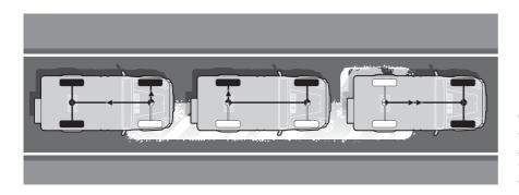
Greater ride stability thanks to 4ETS. If up to three wheels have poor grip, they are braked by 4ETS. The tractive power is then directed to the wheels offering better grip
