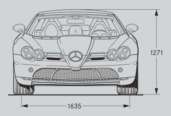
All measurements are in millimetres. The dimensions shown are mean values and apply to standard-specification, unladen vehicles.
