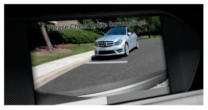
A better view of what's around you. When backing up, the available rearview camera shows a live view of the area just behind your C-Class on the in-dash screen. To help negotiate tight spaces, optional PARKTRONIC's ultrasonic sensors and color LED displays help alert you to nearby objects in low-speed maneuvers. Its Parking Guidance feature displays steering instructions to help you parallel-park the car.
