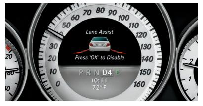
Multilane multitasker. Optional Active Lane Keeping Assist uses a camera to monitor the car's position in relation to visible lane markings. If you start to drift out of your lane without using a turn signal, it can alert you by vibrating the steering wheel. If you disregard the system's alerts, its advanced active technology can also gently apply the brakes to individual wheels, to help draw the vehicle back into its original lane.
