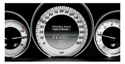
A watchful eye when's it time for a rest. ATTENTION ASSIST® is a Mercedes-Benz innovation that can alert you if it detects signs of drowsiness on long drives. It measures more than 70 variables, starting in the first minutes of a drive, to establish a pattern. By continually monitoring a variety of driving behaviors along your trip, it can offer a warning tone and encourage taking a rest if it senses you're getting drowsy.<sup>8</sup>
