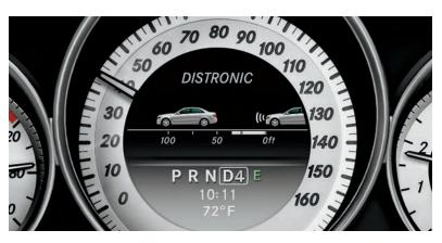
Cruise control that stops and goes. Available DISTRONIC PLUS® uses radar to adapt your set cruising speed in response to the flow of traffic ahead. It can slow the vehicle automatically—or brake to a full stop—then resume with a tap.6 Even if you're not using cruise control, PRE-SAFE® Brake can alert you to stopped traffic, and automatically apply up to 100% braking force to help prevent or reduce the severity of an impact.7
