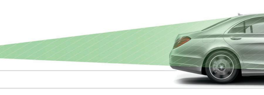
As soon as the driver presses the brake pedal, Adaptive Brake Assist adjusts the brake force.  If the driver brakes, but not hard enough to avoid a collision, the system increases braking force. If the driver does not brake at all in response to the alert, the system can initiate braking autonomously.
