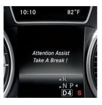
A watchful eye if it's time for a rest. ATTENTION ASSIST® is a Mercedes-Benz innovation that can alert you if it detects signs of drowsiness on long drives. Starting in the first minutes of a drive, the system measures more than 70 variables, to establish a pattern and determine the warning thresholds. By continually monitoring a variety of driving behaviors along your trip, ATTENTION ASSIST can offer a warning tone and encourage taking a break if it senses you're getting drowsy?
