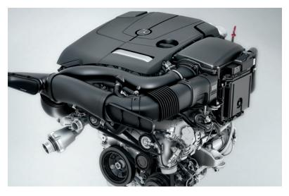
Mileage master. State-of-the-art clean diesel technology makes the GLK 250 BlueTEC® one of the most fuel-efficient luxury SUVs. Two turbochargers—a fast-acting unit for low rpm and a larger, more powerful turbo as the revs build, turn the 2.1-liter inline-4 into a torque-wielding giant: 369 lb-ft comes on at just 1,600 rpm. So in addition to its amazing 24/33 mpg (city/highway)¹, it can thrust you from 0 to 60 mph in 7.8 seconds.³
