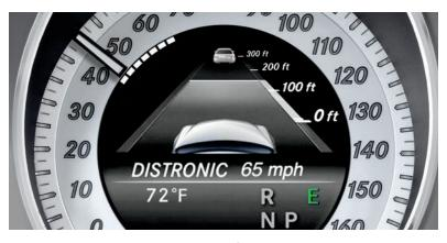
Cruise control that stops and goes. DISTRONIC PLUS® adaptive cruise control uses radar to adapt your set speed in response to the flow of traffic ahead. It can slow the vehicle automatically—or brake to a stop—then resume with a tap. Even if you're not using cruise control, PRE-SAFE® Brake can alert you to stopped traffic, and automatically apply up to 100% braking force to help prevent or reduce the severity of an impact.
