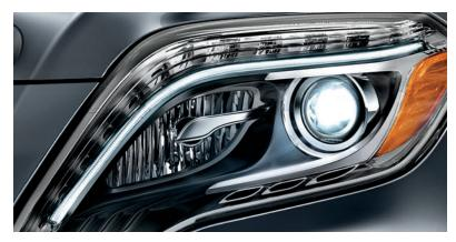
Brighter by day, and by night. The Daytime Running Lamps, rear turn signals, brake lamps and taillamps all feature LED technology. With the Lighting Package, Bi-Xenon headlamps generate light that more closely resembles natural daylight. The package includes Active Curve Illumination and Adaptive Highbeam Assist, both of which continuously vary the beams to maximize illumination without creating glare for other drivers.
