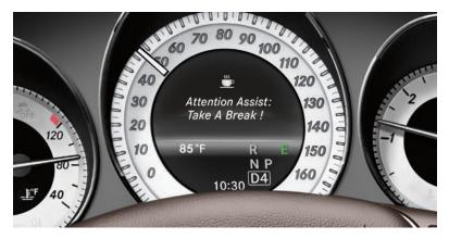
A watchful eye when's it time for a rest. ATTENTION ASSIST® is a Mercedes-Benz innovation that can alert you if it detects signs of drowsiness on long drives. It measures more than 70 variables, starting in the first minutes of a drive, to establish a pattern. By continually monitoring a variety of driving behaviors along your trip, it can offer a warning tone and encourage taking a rest if it senses you're getting drowsy?
