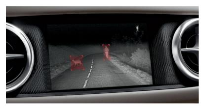
**Nighttime enlightenment.** Available Night View Assist PLUS<sup>6</sup> projects infrared beams that are invisible to the human eye, and reads them with a special camera. It displays a supplemental view of the road on the in-dash COMAND<sup>®</sup> screen, highlighting pedestrians and some animals. A focused flash of the headlamps helps alert pedestrians. You can also set the display to turn on only when it senses a pedestrian or animal.<sup>10</sup>
