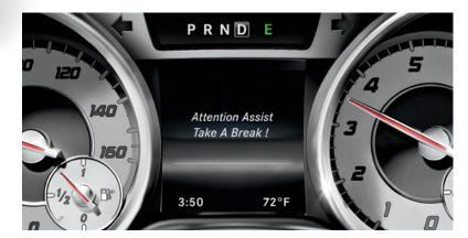
A watchful eye when it's time for a rest. ATTENTION ASSIST® is a Mercedes-Benz innovation that can alert you if it detects signs of drowsiness on long drives. It measures more than 70 variables, starting in the first minutes of a drive, to establish a pattern. By continually monitoring a variety of driving behaviors along your trip, it can offer a warning tone and encourage taking a rest if it senses you're getting drowsy.
