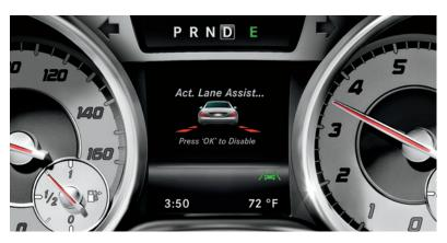
Multilane multitasker. Available Active Lane Keeping Assist<sup>6</sup> uses a camera to monitor the car's position relative to visible lane markings. If you start to drift out of your lane without using a turn signal, it can alert you by vibrating the steering wheel. If you disregard the system's alerts, its advanced active technology can also gently apply the brakes to individual wheels, to help draw the vehicle back into its original lane.<sup>2</sup>
