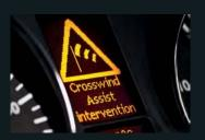
Crosswind Assist<sup>3</sup> can gently engage individual brakes to quickly help stabilize your Sprinter Van and boost safety in strong, gusting crosswinds. This standard feature helps ensure your vehicle remains in its lane at highway speeds.
