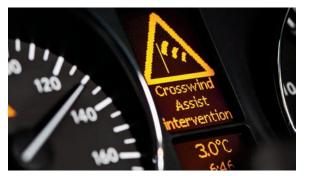
Crosswind Assist<sup>2</sup> can gently engage individual brakes to help quickly stabilize your Sprinter Van and boost safety in strong, gusting crosswinds. This standard feature helps ensure that your van remains in its lane at highway speeds.
