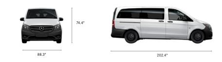
All measurements in inches. All width measurements include mirrors. See page 30 for a complete listing of models and specifications.
