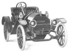
ood looking I-beam front axle; start crank held vertical; lamps
