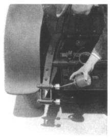
A few moments with an ordinary pump oil can fills the new type wick-feed oilers -their action is then automatic.
