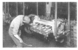
An ingenious check for perfect alignment of connecting rods, pistons and pins before putting on block.
