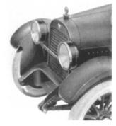
Deep crown fenders with full aprons give complete protection. Radiator shutters and motometer insure motor efficiency and economy.
