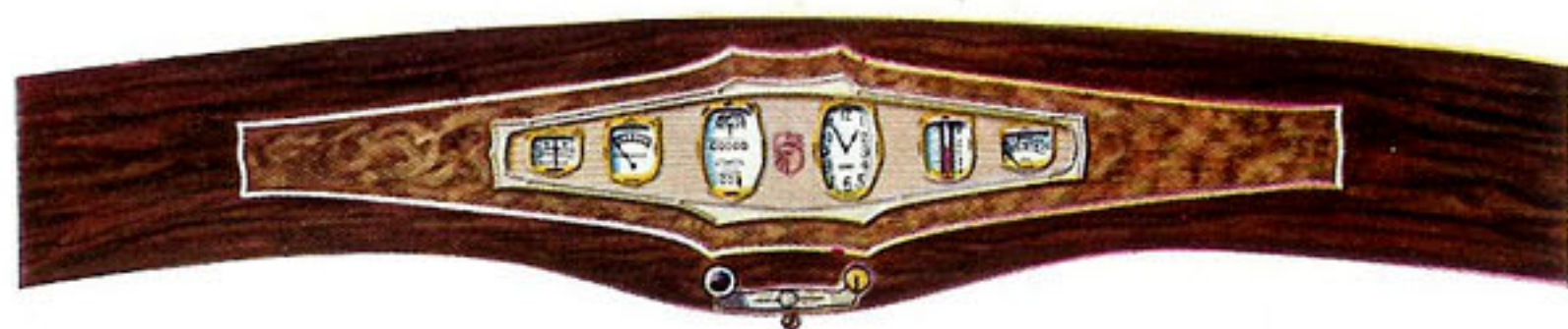
A new design instrument board adds distinction to the Salon interiors of the Advanced Six "400" Series. Fashioned with straight-grain walnut effect, it contrasts smartly with the knurled walnut design which sets off the instrument panel with its antique gold background and similarly finished instruments. In the panel is an electric clock, motor heat indicator, hydrostatic gas gauge, ammeter, oil pressure gauge, and speedometer, while the coincidental ignition-transmission lock is located directly below on the instrument board
