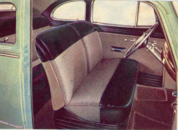
The front seat of the Commodore Club Coupe pivots forward, allowing easy entrance to a rear seat accommodating two extra passengers.
