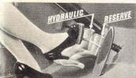
Safest braking system— Two systems in one—hydraulic and mechanical—from the same foot pedal.
