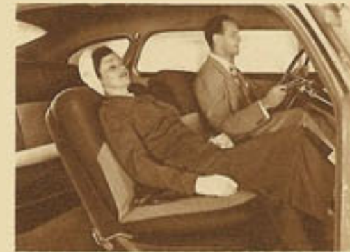
NEW! AIRLINER RECLINING SEAT! Your airliner seat (optional, extra cost) offers five comfortable positions. There's a curved, undivided windshield, exclusive in Nash on all models. The new exclusive glove-locker pulls out instead of spills out. And all dials are clustered in the Nash Uniscope for safety and convenience.
