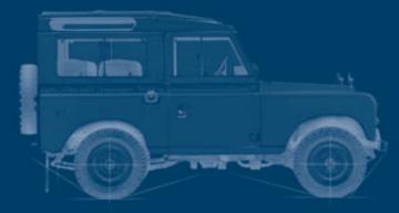
Series III Station Wagon (1972–1984) 1972 Air intake on wing for heater added.
