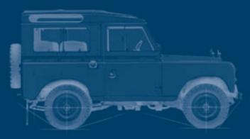
Series IIa Station Wagon (1961-1972) 1966 Electrical indicators become standard. 1968 Headlamps moved from radiator grille to wings.
