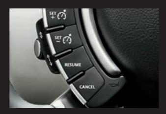
The Adaptive Cruise Control System can be programmed to one of four settings of between a 1.0 second and 2.2 seconds interval from the vehicle in front in normal driving conditions or when Grass, Gravel, Snow is selected on the Terrain Response® dial.
