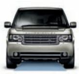
Obstacle Clearance Ground clearance off-road height 11.1 inches (283mm) (Standard ride height 9.1 inches (231mm))
