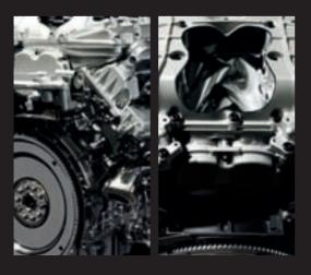
The new LR-V8 Engines feature 'drive by wire' throttle control and camshaft profile switching to increase torque and improve performance.
