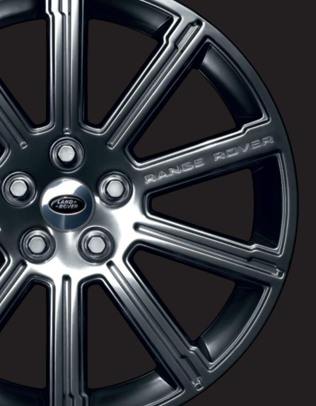
The new 2010 Range Rover's alloy wheels are manufactured from extremely resilient material. They are designed to enhance the vehicle's appearance as well as improve handling by reducing unsprung weight, allowing the suspension to react more quickly. Not only has each one been through a series of formidable tests, to simulate on-off-road stresses, every individual wheel is also x-ray checked by the wheel manufacturer.
