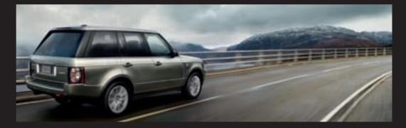
Enhanced Understeer Control uses the new 2010 Range Rover's technologies to increase stability and help improve safety. The system recognizes when the vehicle is travelling too fast to smoothly negotiate a corner, by reducing engine torque and, if necessary, applying the brakes to the appropriate wheel. Land Rover encourages drivers to practise safe driving conditions when towing a trailer.
