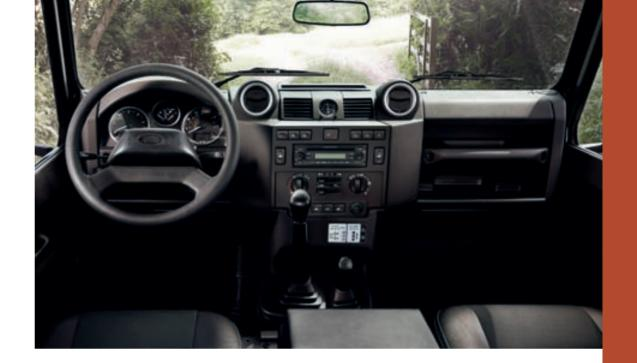
Form follows function in the Defender interior. Tough vehicles demand robust materials such as the scuff-resistant facia and durable seat coverings. The facia is a one-piece moulding for improved refinement, its distinctive lines providing Land Rover's traditional commanding view of the ground ahead.
