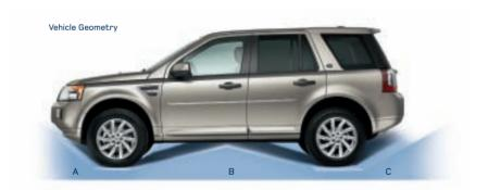
A Approach Angle 29° B Ramp Break Over Angle 21.5° C Departure Angle 32°
