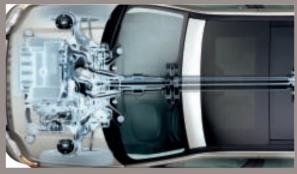
PERFORMANCE WITH REFINEMENT A compact, advanced 3.2 liter straight-six engine with Cam Profile Switching and Variable Valve Timing delivering more power, a better spread of torque and greater efficiency.
