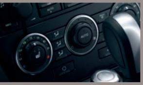
**CLIMATE CONTROL** Standard air-conditioning system with dual-zone climate control, with pollen filter and humidity sensor maintaining fresh air in the cabin, keeping you and your passengers comfortable.
