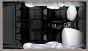
SAFETY Ultra-high-strength steel is used to construct an immensely strong monocoque body and inner safety cell protected by front and rear energy absorbent crumple zones. Seven airbags are fitted as standard on all vehicles.
