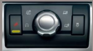
**TERRAIN RESPONSE®** Land Rover's patented Terrain Response® system adds to Land Rover LR2's breadth of capability. Any of the four settings — general driving, grass/gravel/snow, mud and ruts, or sand — can be easily selected by simply turning the rotary control. In addition all vehicles with Terrain Response® are also fitted with Hill Descent Control and Land Rover's Gradient Release Control systems.
