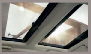
PANORAMIC SUNROOF The standard panoramic sunroof — with a fixed rear section and electric tilting/sliding front section — adds to the feeling of lightness and airiness within the cabin. The glass is specially formulated to filter the sun's infrared rays, providing light without unpleasant heat. Both sections also include a convenient blind
