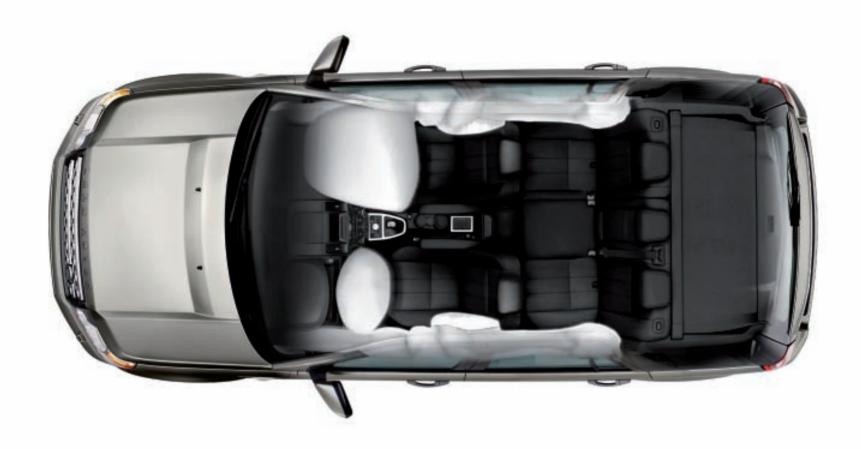
Getting tough with safety. The immensely strong monocoque body and inner safety cell, protected by meticulously engineered front and rear crumple zones, absorb energy on impact. While ultra-high-strength steel is used in the construction of the body, dual-phase steel, which requires special pressing because of its resilience, is found in key components such as the front windshield pillars and lower side sills. The result is a first class, weight-efficient safety cell.
