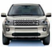
Front Axle Clearance Ground clearance up to 8.3 inches/211mm
