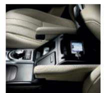
The Portable Audio Interface includes a 3.5mm auxiliary socket, USB port and dedicated iPod® connection.
