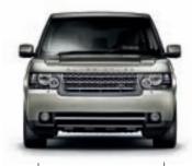
Height 73.9 inches/1,877mm Standard height includes satellite antenna Front wheel track 64.1 inches/1,629mm Access height air suspension setting reduces height given by 1.6 inches/40mm to 72.3 inches/1,837mm
