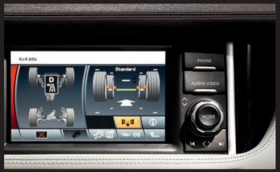
Terrain Response uses a rotary dial on the center console (and grouped in a convenient cluster with the air suspension height control, Hill Descent Control with Gradient Release Control (GRC) and the High/Low Range selector) to choose settings for different driving environments.
