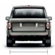
Rear wheel track 64 inches/1,625mm Width 80.1 inches/2,034mm mirrors folded Width 87.2 inches/2,216mm mirrors out
