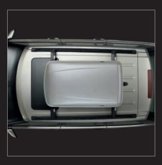
Luggage Box\* VPLDR0003 Lockable for security. Opens from both sides. External dimensions: 63 inches long, 37 inches wide, 16.1 inches high. Volume 118 gallons. Load capacity 132.3lbs.
