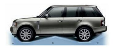
A Approach Angle Standard ride height 29 (22.9) \*, off-road 34.0 (25.4 )\* to spoiler with air suspension raised
