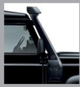
Raised Air Intake LR008383 Full Coloured Union Jack - LR027664 Ideal for dusty conditions, this raised air intake secures to the vehicle's 'A' post and also utilises the existing air intake vent fixings. Suitable for Td5, 2.4 and current 2.2 Diesel engines.
