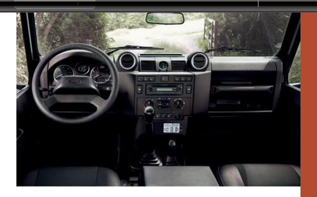
Form follows function in the Defender interior. Tough working vehicles demand robust materials such as the scuff-resistant facia and durable seat coverings. The facia is a one-piece moulding for improved refinement, its distinctive lines providing Land Rover's traditional commanding view of the ground ahead.
