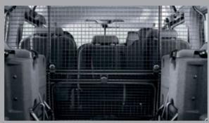
Designed to prevent cargo and luggage from entering the passenger compartment. Manufactured in black nylon coated steel and easy to remove when not required.
