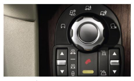
TERRAIN RESPONSE® SYSTEM†. Standard on every Land Rover LR4 and optimizes the vehicle set-up for virtually all on-road or off-road driving situations, with five different settings to suit different terrains such as Grass/Gravel/Snow, Sand, Mud and Ruts and Rock Crawl.
