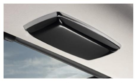
WHITEFIRE®. This technology is a wireless system, discreetly housed in a unit in the vehicle's headlining, which allows the convenient use of cordless headphones with the optional rear seat entertainment system.
