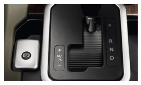
ELECTRIC PARKING BRAKE (EPB). A lever is located next to the gear selector to electrically apply and release the parking brakes on the rear wheels. A simple pull of the lever applies the brake manually and a press releases it. The parking brake will also release automatically upon drive away.
