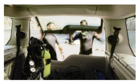
SPLIT TAILGATE. Make light work of difficult loads with Land Rover LR4's two-piece, asymmetric tailgate design. Both upper and lower tailgates are made from resilient lightweight aluminum. The tailgate gives impressive access to the rear of the vehicle and comes into its own when loading large, bulky or heavy objects. The asymmetric portion of the lower tailgate provides a reduced reach-in distance when open and a lower load height when closed.
