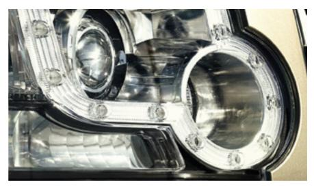
AUTOMATIC HEADLAMPS WITH HIGH BEAM ASSIST\*. Detect vehicle headlamps/tail lights and dip the high beam until the light source is out of range. The system is able to distinguish between automotive and non-automotive light sources.
