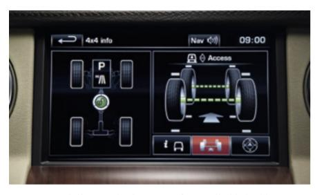
AIR SUSPENSION. Standard four-corner independent air suspension features variable ride height and electronic cross-linking for a constant level ride height irrespective of passenger load distribution. Ride height can be raised up to 2.2 inches/125mm to clear obstacles or lowered by 1.9 inches/50mm for easy access and loading.
