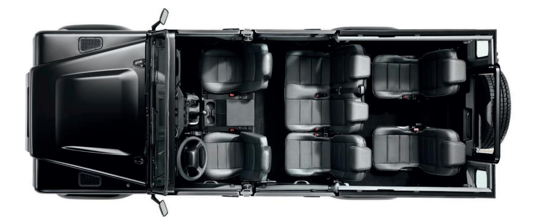
Form follows function in the Defender interior. Tough working vehicles demand robust materials such as the scuff-resistant facia and durable seat coverings. The facia is a one-piece moulding for improved refinement, its distinctive lines providing Land Rover's traditional commanding view of the ground ahead.
