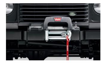
Rated capacity of 9,500lb/4,310kg. 38 metres x 8mm diameter wire rope. This powerful electric winch is designed to fit easily to the front of your Defender, even if the air conditioning option is fitted. Offering maximum reliability for all general winching and self recovery requirements, the winch is available as a complete vehicle kit, ensuring specification and installation are straightforward.
