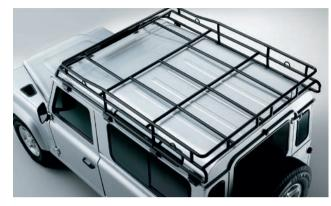
Expedition Roof Rack System<sup>†</sup> VPLDR0063<sup>‡</sup> – 90 Hard Top/Station Wagon VPLDR0064 – 110 Hard Top/Station Wagon (not shown) VPLDR0065<sup>‡</sup> – 110/130 Double Cab (not shown) Heavy duty rack system secured by clamps to the roof gutter.
