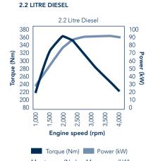
Max torque (Nm) Max power (kW) 360Nm/2,000rpm 90kW/3,500rpm
