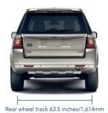
Width 78.9 inches/2.005mm mirrors folded Width 86.4 inches/2,195mm mirrors out
