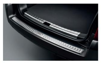
Stainless Steel Rear Bumper Tread Plate VPLFB0040 Stainless Steel Tailgate Latch Finisher VPLFB0039 – (also shown)
