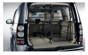
Cargo Divider EOH500040 Separates luggage space into two protected sections. Lockable outer gate on one side. Must be fitted with Cargo Barrier. Not compatible with standard loadspace cover.\*\*
