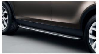
The side steps aid entry and exit to the vehicle and improve access to the roof. Design features include bright stainless steel edge trim and a rubber tread mat.
