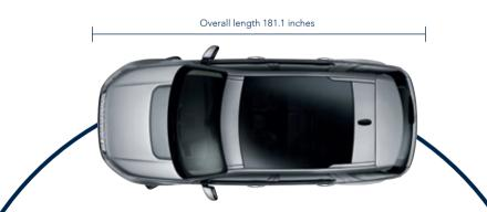
Turning Circle Curb-to-curb 38.1 ft Wall-to-wall 38.9 ft Turns lock-to-lock 2.31
