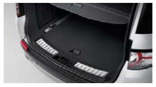
Rear Cargo Space Treadplate Finisher VPLCS0353LAA – Lunar VPLCS0353PVJ – Ebony (not shown) Manufactured from stainless steel with a Bright finish, the rear cargo space treadplate finisher provides protection for the cargo space trim when loading or unloading.
