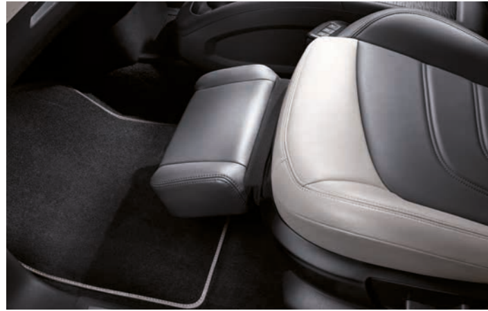
Front passenger's seat: electric footrest
