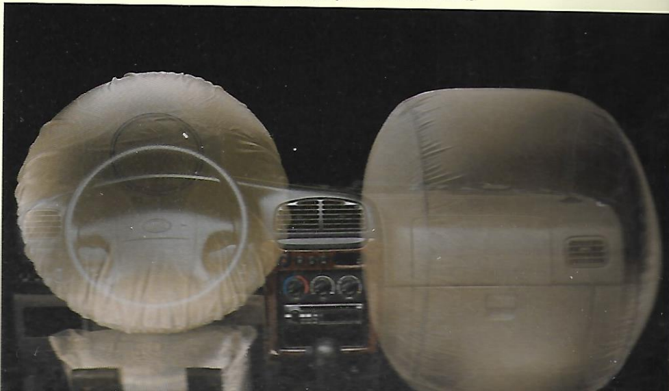
Dual front airbags and driver's knee airbag are standard features on both models.**
