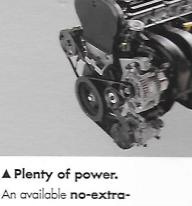
An available no-extracharge 2.4-liter DOHC 16-valve four-cylinder engine delivers a healthy 150 horsepower.
