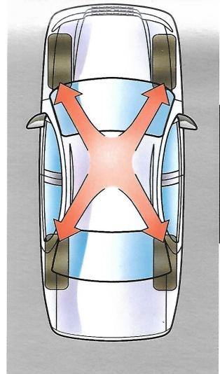
the-corners design and cab-forward architecture result in more stable handling, more interior room and wider door openings.
