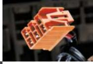
TRAILER-READY. The trailer-ready design of Silverado features an eight-wire lead along with an available seven-pin connector and weight-distributing hitch (included with the Z82 Heavy-Duty Trailering Package).
