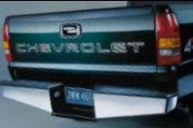
REAR BUMPER. This drop center bumper features a non-skid step pad and a 500-lb. tonaue weiaht
