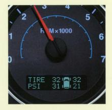
The Tire Pressure Monitoring System notifies you if any tire loses air pressure. The available display system (shown) transmits individual tire pressure.
