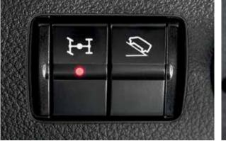
Activated at the push of a button, the Sprinter 4x4 uses 4-ETS® to control individual wheels, instantly providing ground-gripping power.
