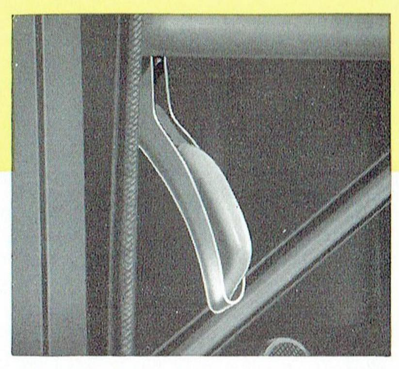
The parking brake lever is the inverted type. It is mounted in back of the instrument panel, to the left of the steering column. In this location it is out of the driver's way yet convenient for him to reach.
