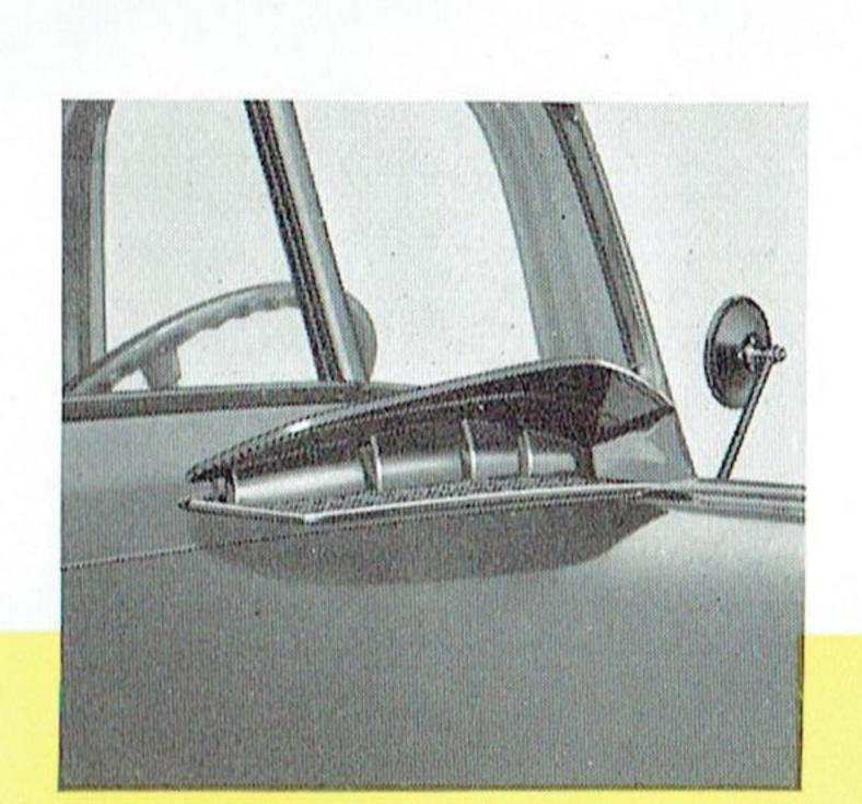
The cab on Regular Trucks is equipped with a large screened ventilator. A friction device holds it in any position. Cowl ventilators on C.O.E. cab are illustrated on Page 7.
