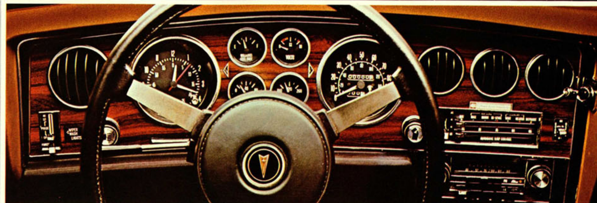
The instrument cluster is straight out of Grand Prix. Custom Sport steering wheel and rally gauges are available.
