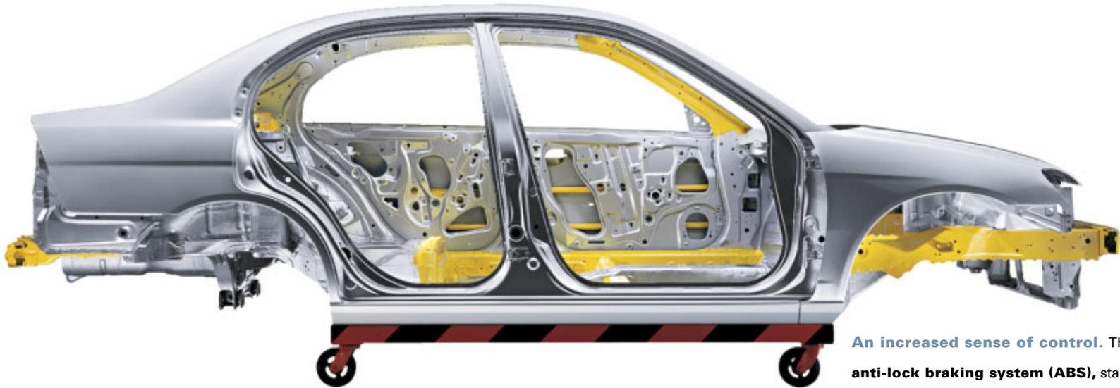
**An increased sense of control.** The Honda-built **anti-lock braking system (ABS)**, standard on EX models, pulses brake-line pressure many times per second. This allows the driver to retain steering control when braking hard on wet or slippery roads.
